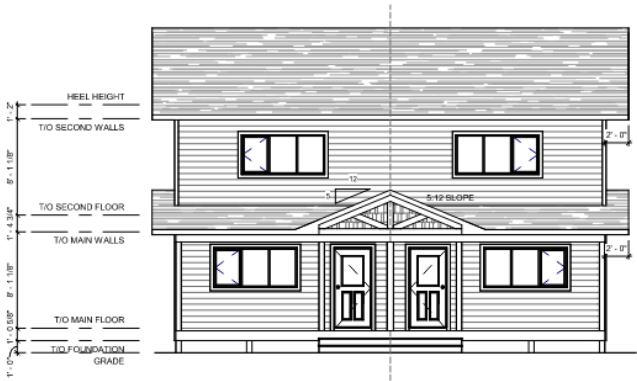
FRONT ELEVATION SCALE 1/8" = 1'-0"
